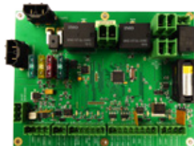
Emergency vehicle lighting mast control
