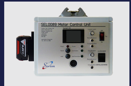
Test equipment powered by a tool battery using SEL0092
