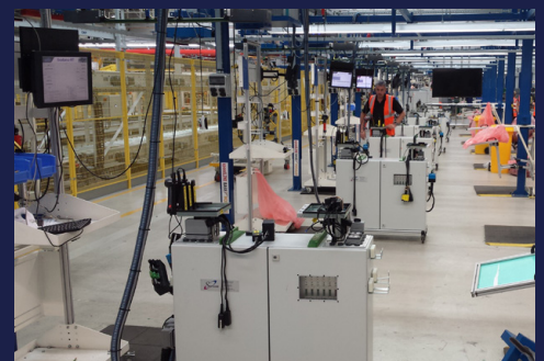
End of Line Test Stations
