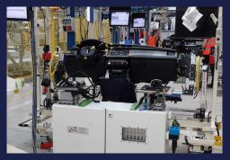
Automotive cockpit end of line test stystem
