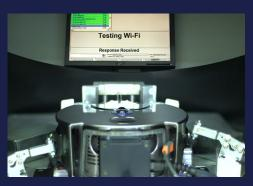
Robotic vacuum cleaner test and calibration
