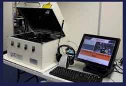
Vehicle air distribution unit (ADU) end-of-line test
