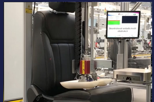
The force unit applies a predetermined load pressure
