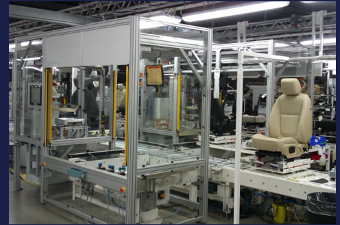
FAMs can correctly test the operation of an ODS (IEE) mat
