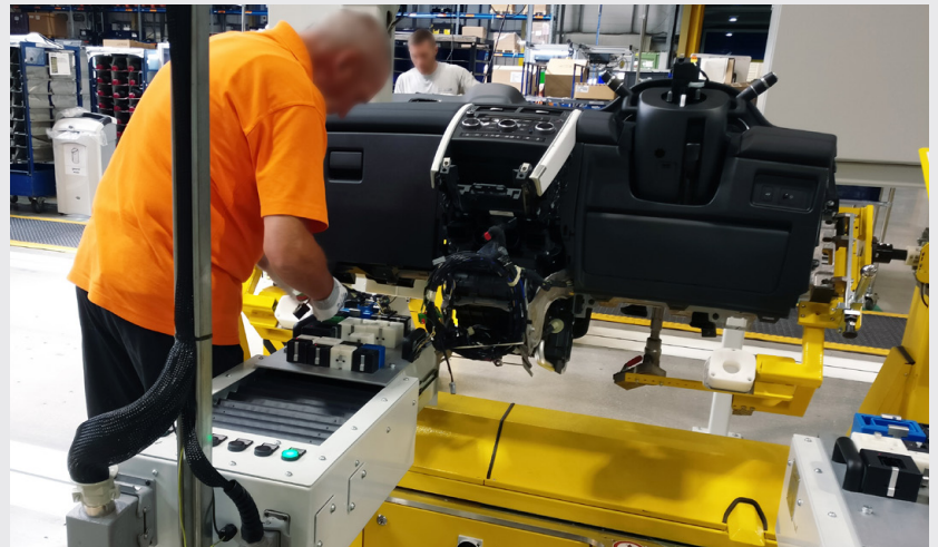
End of line test station at IAC Halewood
