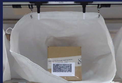
Bags are attached to the rack using a hooking method for quick removal
