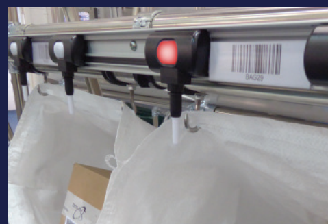
The lights indicate where the items need to be placed
