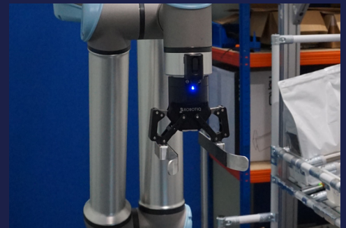
The picking robot is fitted with a gripper to pick up bags
