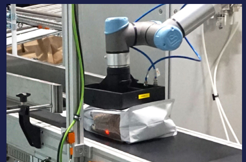
The labeling robots are fitted with a bespoke label application head
